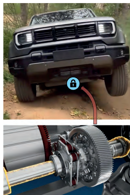
Fig. 3 An off-road SUV equipped JJE eLocker in both front and rear drive unit
