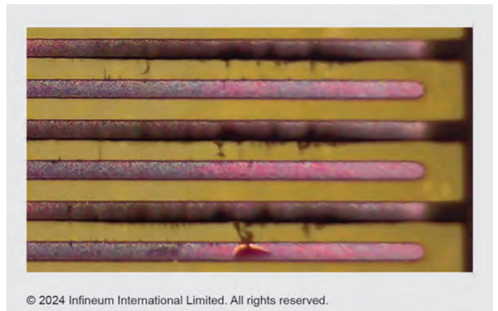
Fig. 4 Deposit / dendrite growth between anode and cathode
