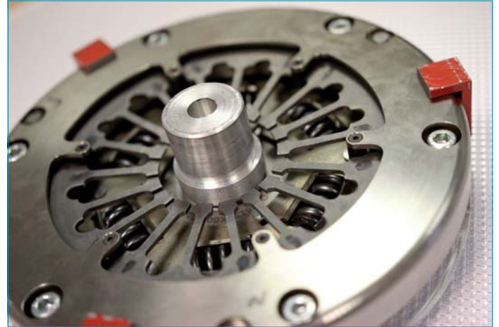
Figure 2 Unlike a manual clutch and transmission, there is a substantial inertia on either side of a hybrid disconnect clutch
