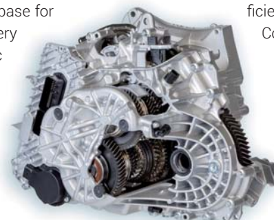
Figure 1 Dual-clutch transmission 7DCT300 with wet dual clutch, electrohydraulic clutch actuation and electromechanic shift actuation
