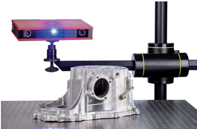
Figure 2 The new 3D optical scanner offers Goudsmit a whole new level of measurement technology and deliver three-dimensional measurement data and analysis for industrial and automotive components.
