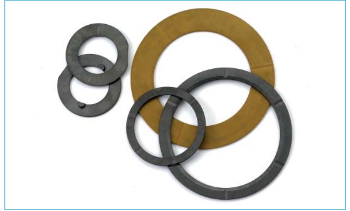
Figure 3: Transmission parts such as thrust bearings are increasingly being made of high-performance plastics such as PAI and PEEK instead of metal for light weight, design flexibility, improved wear resistance, and space savings.
