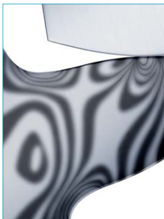
Figure 1: Complex gear loading yielding a contact stress on the flank and bending stress in the root.
