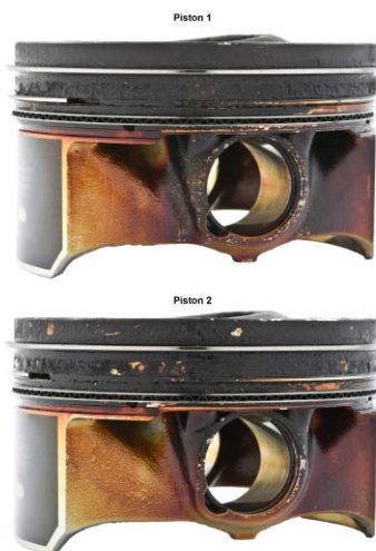
Figure 5 Hot Stuck Piston Rings
