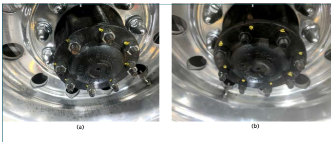
Figure 20 iLok™ nut installed on both trucks after the tests. (a) Phosphate coated parts installed on a 2011 model truck, (b) zinc coated parts installed on an OEM test truck
