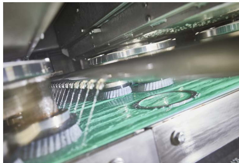
Automated planetary brush deburring/surface preparation process
