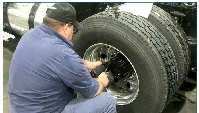
Figure 21 Mechanic removing the iLok™ nut. One tool used and less than five minutes needed to remove all eight nuts and pull the shaft off the hub.
