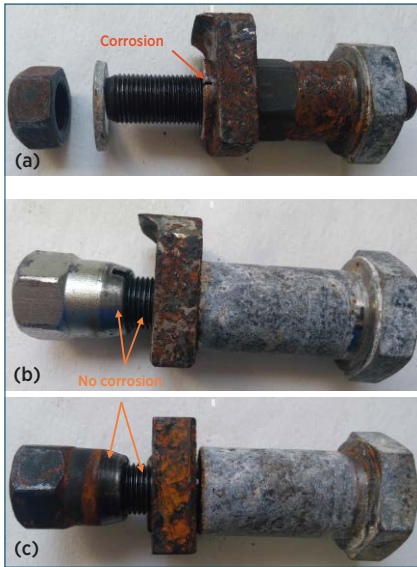
Figure 19 Parts after 72 hours of salt spray: (a) 3-piece system, (b) iLok™ nut zinc coated, and (c) iLok™ nut phosphate coated
