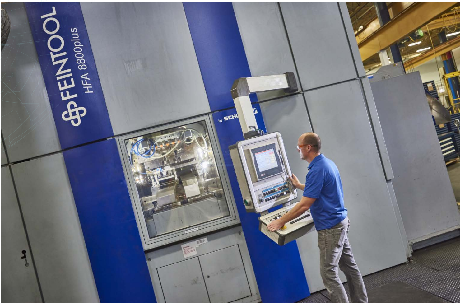
FineClutch fineblanking tool installed in a 880 ton Feintool Fineblanking Line
