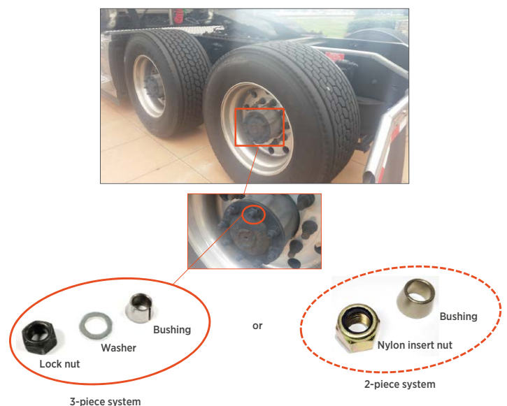
Figure 1 3-piece and 2-piece fastening systems used on rear axle hub assemblies.
