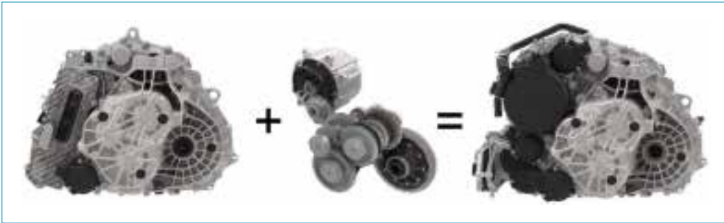
Figure 5 Torque-split hybridisation for dual-clutch transmissions (7DCT300 to 7HDT300)
