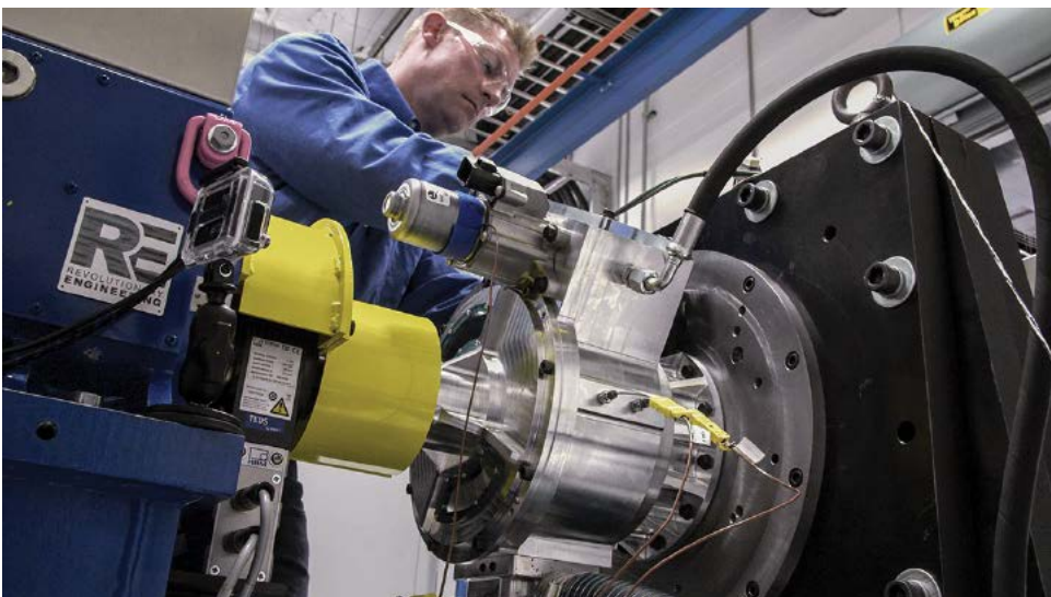
With more than 70,000 hours of durability testing accumulated on the core technology, the VariGlide® variator presents OEMs with a durable, fuel-efficient, beltless CVT technology.
