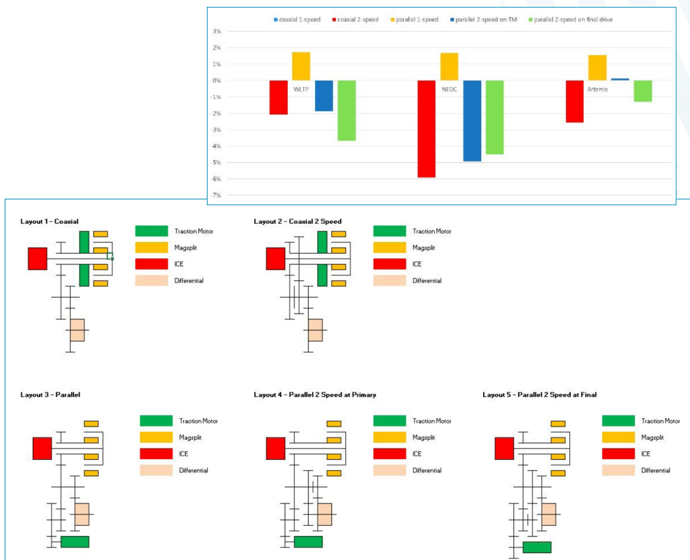
Figure 3 Relative fuel consumption vs transmission arrangement
