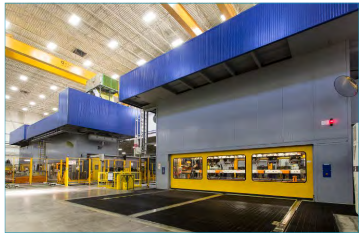
Figure 3 Feintool Nashville has three large transfer press lines with the newest 1,600 direct servo press in the front.
