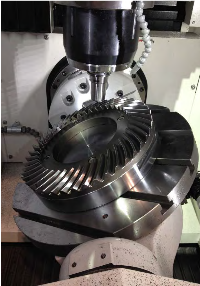
Figure 5 Hardmilling of Spiral Bevel Gear Carburized to 55 HRC on MazakVC500 5X
