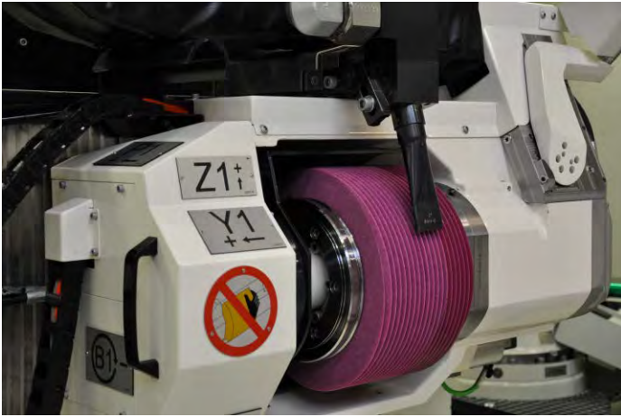
Figure 4 Two-zone grinding worm (Grinding & Polishing)
