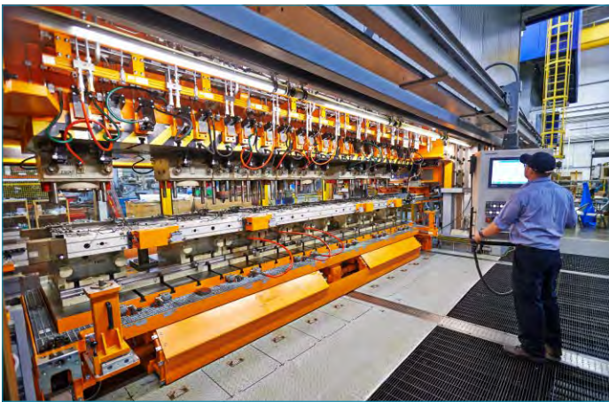
Figure 2 On a large 18-foot press table with moving bolster, components can be finished in up to 12 tooling stations in a single transfer run.
