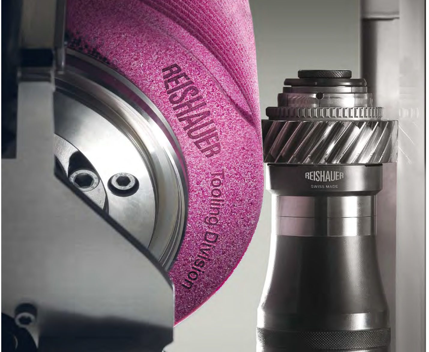
Figure 1 Continuous generating gear grinding
