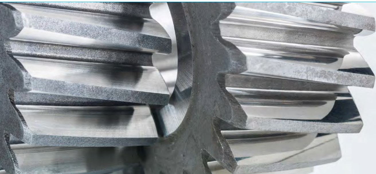
Figure 5 Ground and polished gear flanks
