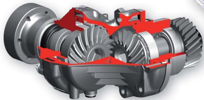
The power take-off unit of the new 4MATIC powertrain
