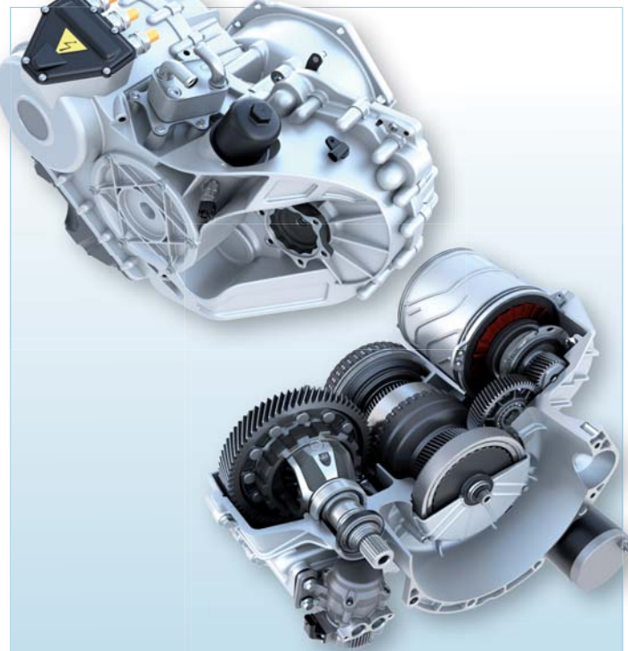
Figure 5 Future Hybrid transmission design with axe-parallel EM integration
