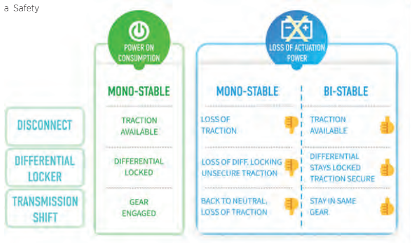
Figure 5: Advantages of Bi-stable Electromagnetic Clutch
