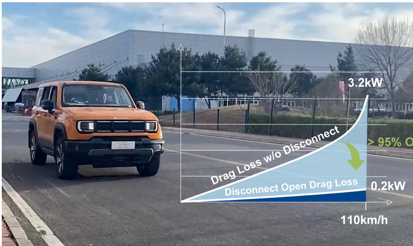
BJ40e Test Vehicle with JJE's DL Combo™ Differential & Drag Loss Chart
